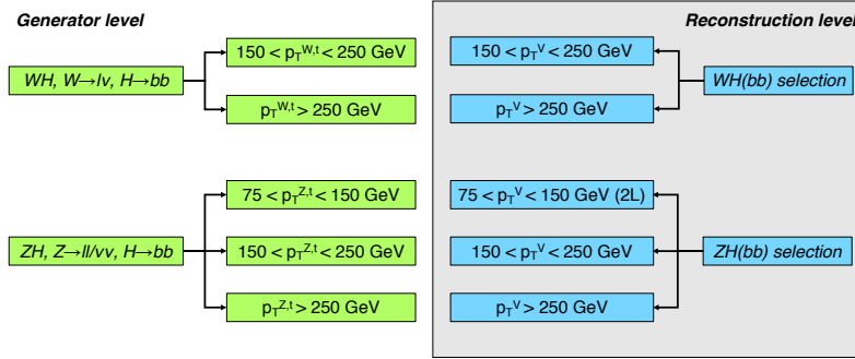
Figure 1: The simplified template cross-section regions used for measurements and the corresponding reconstructed VH, H \rightarrow b\bar{b} analysis regions. The analysis is not sensitive to the regions WH, p_T^{W,t} < 150 GeV and ZH, p_T^{Z,l} < 75 GeV, and their cross-sections are fixed to the SM prediction within their theoretical uncertainties. All leptonic decays of the vector bosons (including Z \rightarrow \tau\tau and W \rightarrow \tau\nu , which are extrapolated from the electron and muon channel measurements) are considered for the STXS definition.
