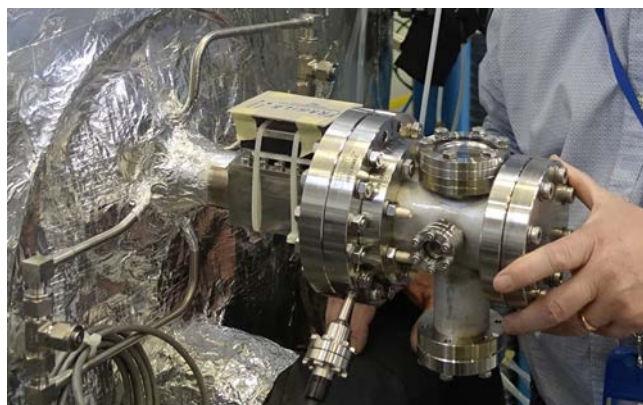
Fig. 8: The Charged AeRosol Generator (CHARGE) at CLOUD14, Nov 2019. CHARGE comprises an electro-spray charged aerosol source followed by an X-ray section before entering the CLOUD chamber. The aerosol particles are neutralised when the X-ray source is switched on, allowing an experimental comparison to be made between charged and uncharged aerosol particles. Optical ports on CHARGE allow visual confirmation of proper operation of the electro-spray tip.
