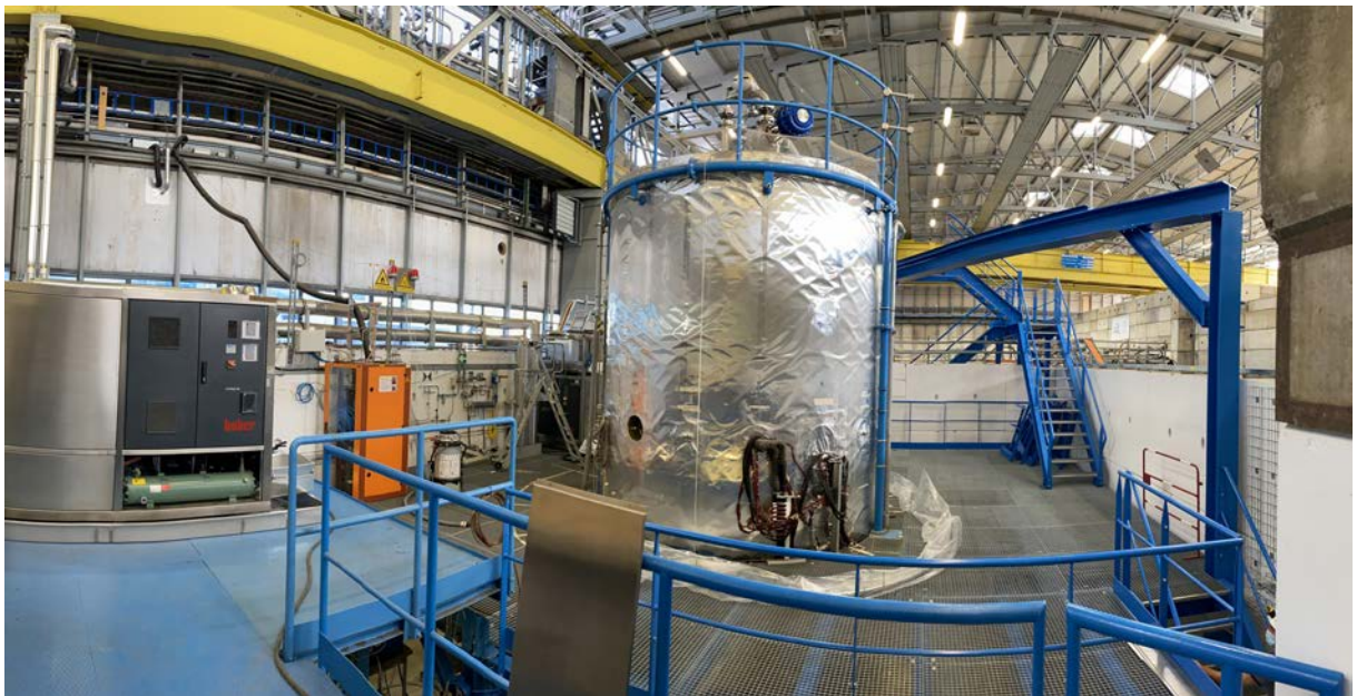
Fig. 9: Model drawing of the East Area T11 zone and CLOUD facility when completed. Model drawing of CLOUD in the T11 experimental zone at the CERN Proton Synchrotron after completion of the East Area renovation, 2019–2021. In addition to the new T11 beamline, essentially the entire CLOUD facility infrastructure, gas system and controls systems will have been rebuilt by the end of 2021.
