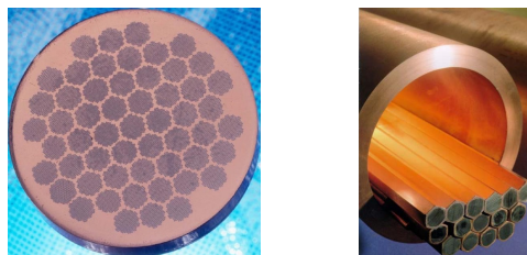
Fig. 15: Nb-Ti wires; left: Cross section of a wire, right: Nb-Ti billet
