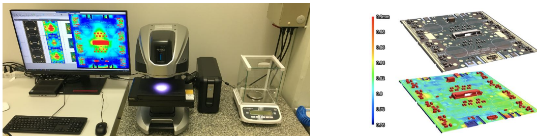
Figure 2. Optical metrology measurement system along with a milligram weighing scale (left) and an example of a 2D scan conducted on an assembled quad module (right).
