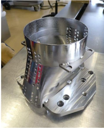
SPS shields after flange assembly
