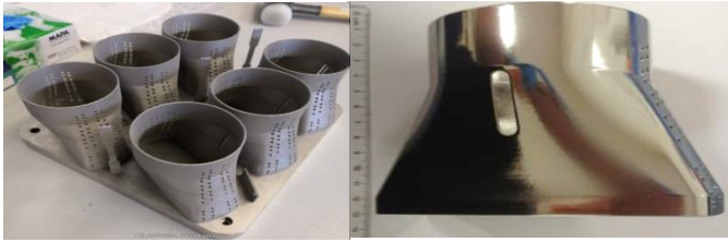
SPS MBB-QD pumping port shields: batch of 6 shields out of the AM machine (left), MBB-QD shield after polishing (right)
