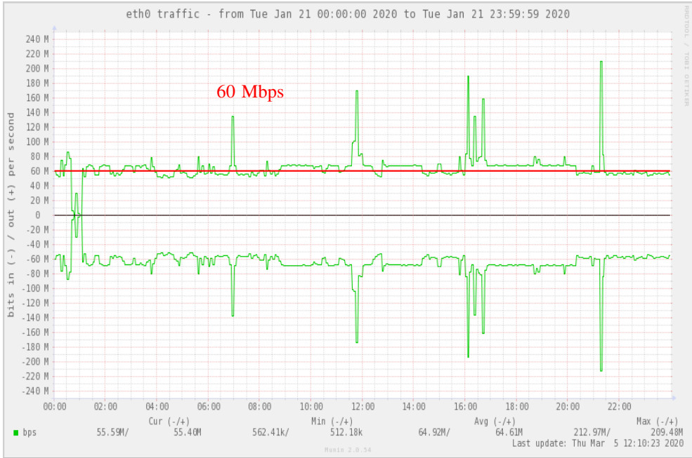
Figure 2. Network performance over 24 hour period with sshfs 2.10. There is network saturation around 60 Mbps.
