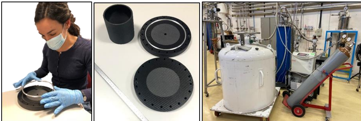
Fig.3 Pipe and flanges with special carbon materials and layout for leaktightness verification at cryogenic temperatures
