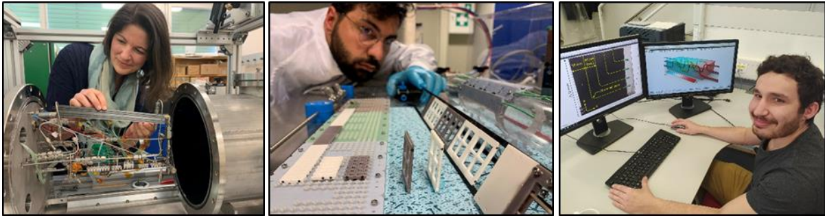
Fig.2 Different on detector microcooling solutions under development and test (left to right, CO 2 test set-up for thin plastic pipes, 3d printed microchannel LEGO, study for microvascular network embedded in a carbon coldplate)
