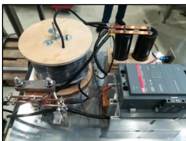
Figure 8. Snubber demonstrator tested at Cryolab.
