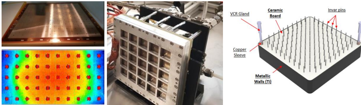
Fig. 2: Top Left: 10cmx10cm micromegas with 100 readout pads. Bottom Left: planarity measurements to monitor and optimize the production processes. Center: prototype under test at the GDD laboratory. Right: Technical drawing of the hermetic prototype.
