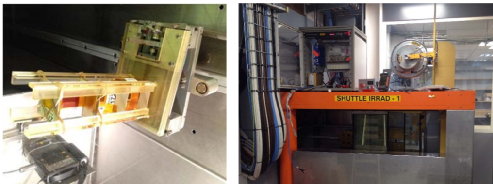
Fig. 1.5.: IRRAD1 Shuttle. Samples holder (left) and loading station (right).
