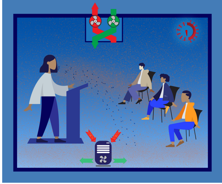
Figure 3: Simplified illustration of the infection model visualising the particle emissions of the infector via i) large size particles that fall quickly on the floor and ii) smaller size particles that spread throughout the volume with low settling velocities in typical indoors environments. The air handling unit on the top represents the renewal with clean outdoor air, the symbol on the top-right corner represents the biological decay of the virus in air and the mechanical device at the bottom represents an air cleaner with HEPA filtration grade.
