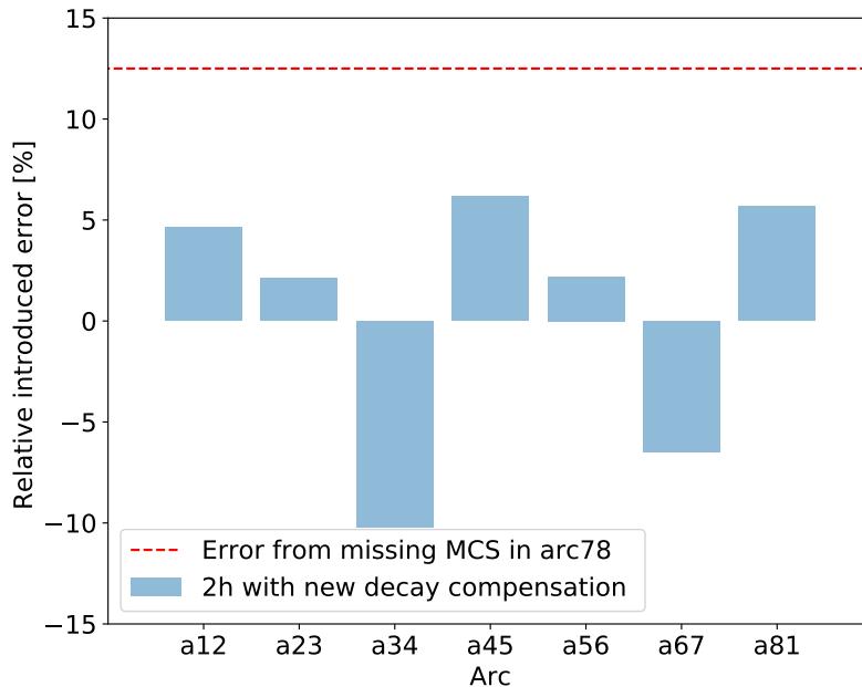
Figure 5: The relative error introduced after 2 h by the uneven knob in percentage of the static local over correction due to the missing MCS in arc78 for Beam 2.
