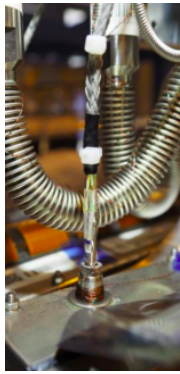
Figure 7.10: PT100 glued onto the dry gas outlet
