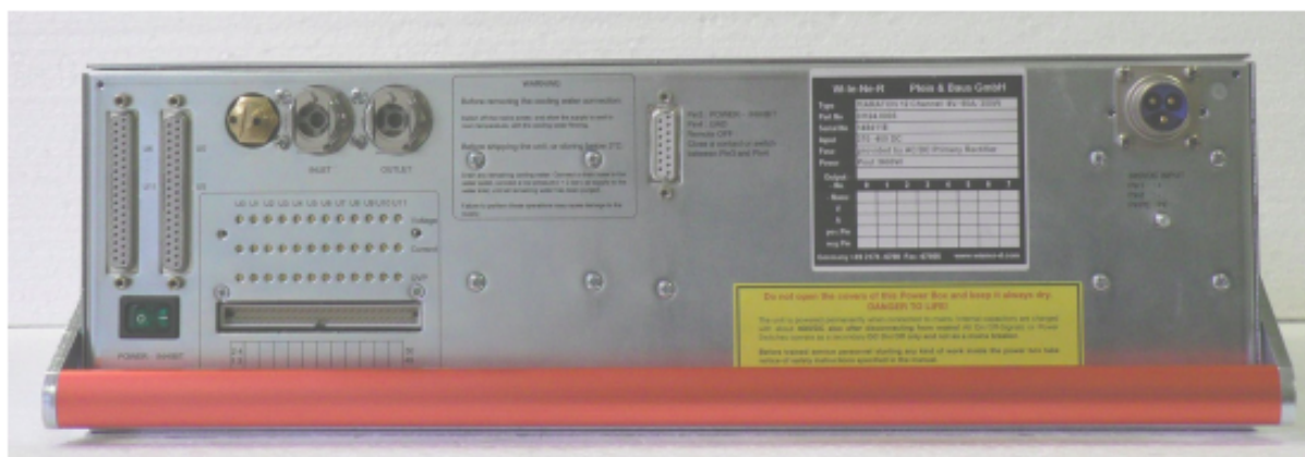
Figure 7.4: Frontal view of a W-IE-NE-R MAgnetic field and RADIation TOLeraNt (Maraton) power supply, developed for the CERN LHC [77].
