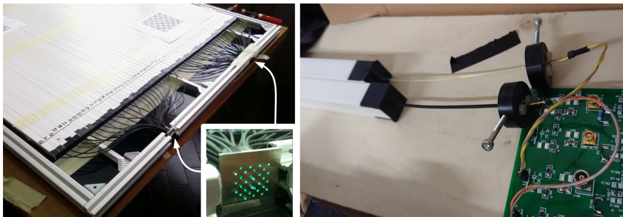
Figure 43 – Left: photo of the current scintillating bar detector internal layout where the WLS fibers are grouped into 2 bundles each one read out by a multi-anode PMT (not shown); right: detail of the experimental setup of the preliminary tests for the read out with SiPMs.
