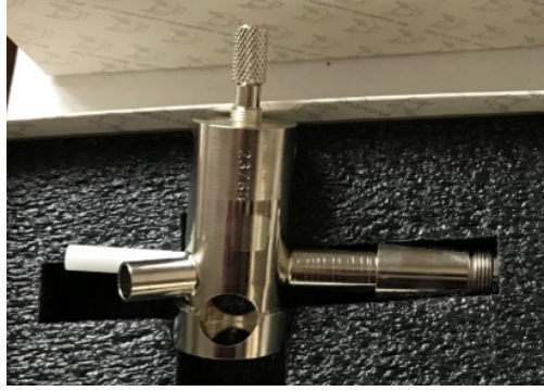
Figure 47 – Evenson cavity that can be installed around a glass tube guiding the molecular hydrogen gas. The tunable cavity is operated at 2.45 GHz.
