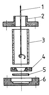
Fig. 1. Schematic of electroplating cell for Pu deposition.
