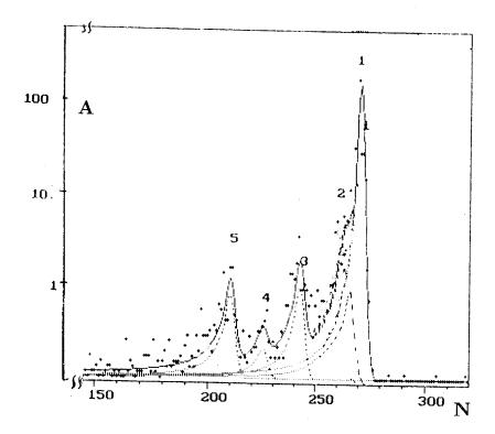
Fig. 2. Alpha-spectrum of a plutonium fraction isolated in Dubna ( see Table 2, sample 2 ).
