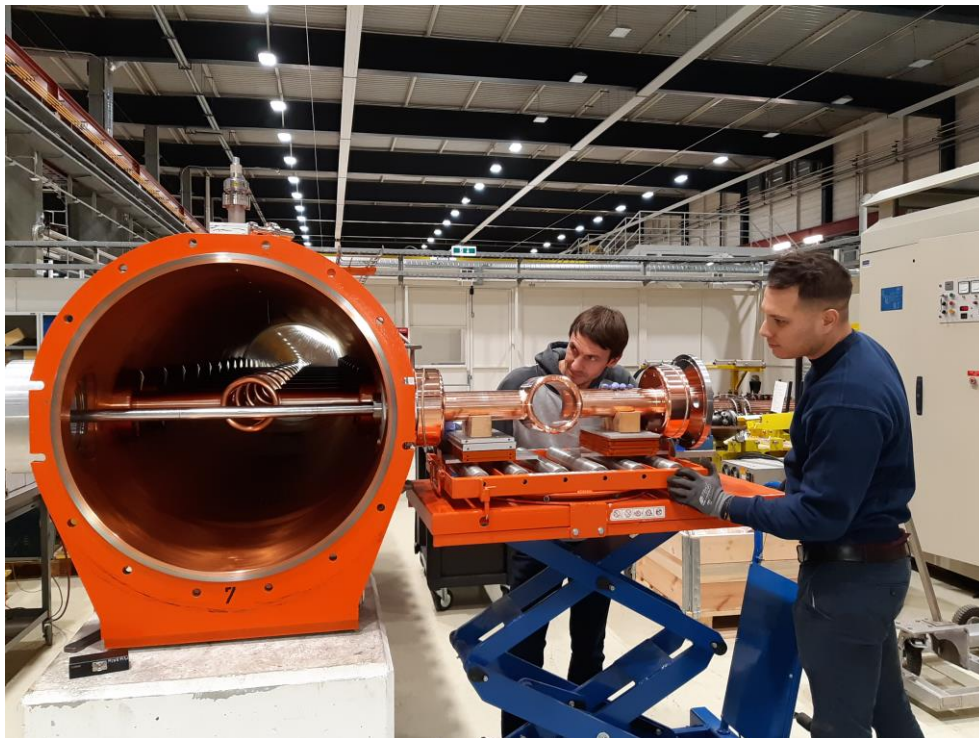
Figure 42. Assembly of new drift tubes for the 200 MHz TWC in building 867.
