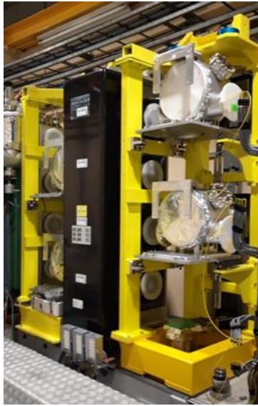
Figure 27. Left: LIU BWS support structures and vacuum tanks installed in the PSB, September 2019. Right: Example of LIU BWS calibration results, showing the residuals of the linear fit between the measured angular position and the projected wire position.
