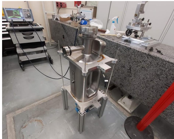
Figure 22. Trim tuning of RFD crab cavities (horizontal crabbing) to ensure they meet the correct frequency in their operational conditions. Tracking and analysis of Higher Order Modes (HOMs) to assess their effect on beam stability and heat-load.
