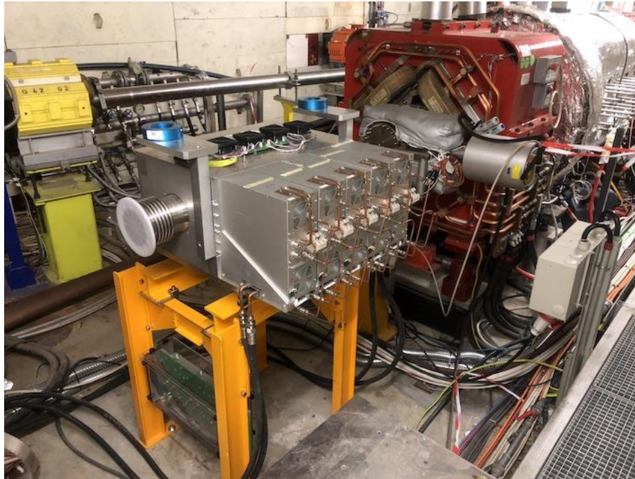
Figure 59. The new C02 cavity in AD, an updated version of the PSB Finemet® prototype.
