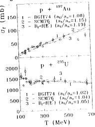
Fig. 6. Incident energy dependence of fission crosssections for proton-gold and proton-uranium interactions. The experimental points are from the summary Table 159 of the monograph [21]. The lines are our CEM calculations performed with different fission barriers (for details see Ref. [26]) for the values of  $a_f/a_n$ shown in the figure.
