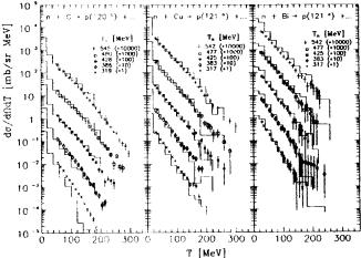
To illustrate the relative role of different proton production mechanisms for neutron-copper collisions at 425 MeV, as an example, the cascade, pre-equilibrium and the evaporative components of proton spectra are shown separately in the upper part of Fig. One can see that the contribution main protons to the spectra comes from the evaporation from com-
