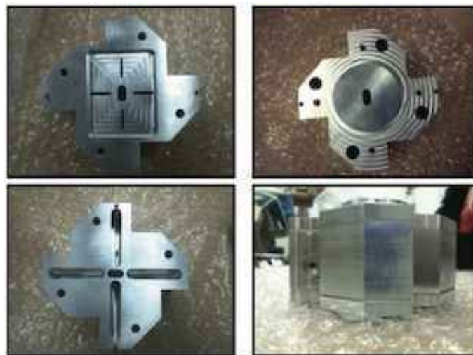
Figure 52: Fabricated one block Low-Q IP-BPM (BPM-C). Sensor cavity part (left up). Wave guide part (left down). Cavity covers with flange (right up). Side view after stacking (right down).
