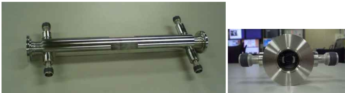
Figure 46: Side view of the stripline kicker
