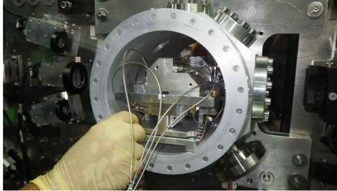
Figure 54: IPBSM installed in the vacuum chamber at IP. BPM is mounted on the mover cradle.
