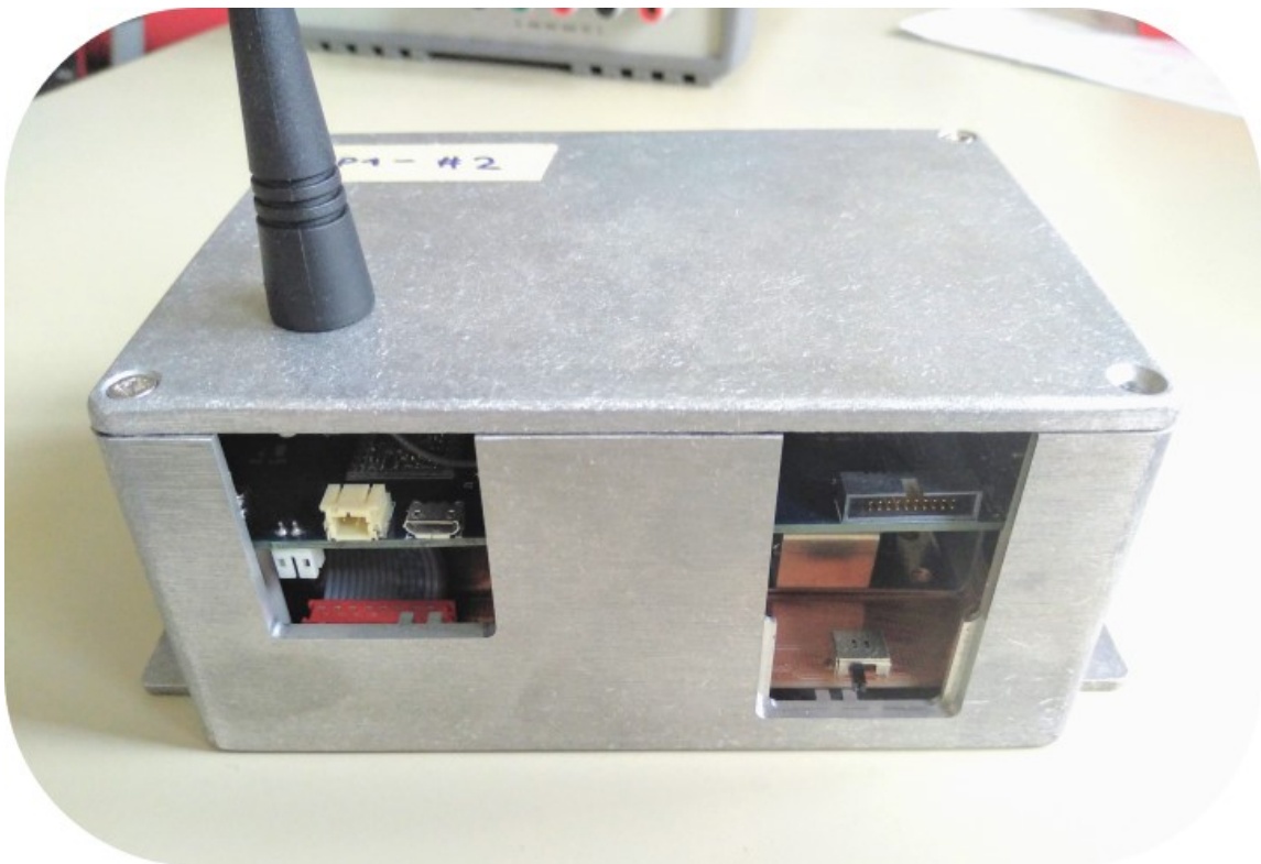
Figure 7.1: An assembled prototype of a BatMon sensor node.
