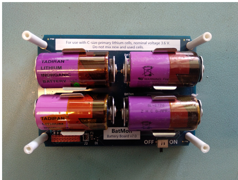
Figure 4.8: Assembled battery board including vertical supports for mounting of the main board
