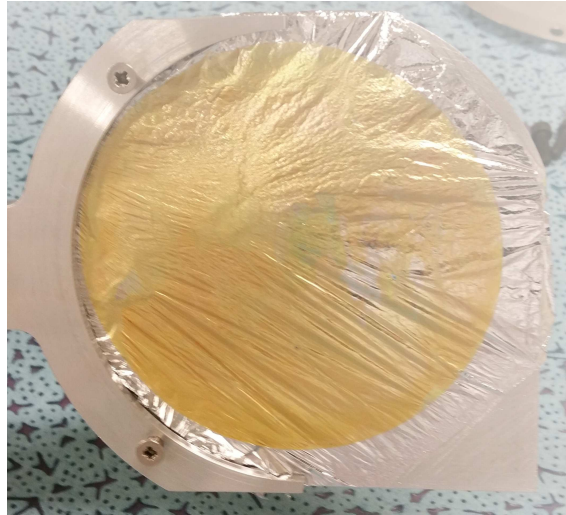
FIGURE 5.11: A photograph of the uranium target used in STEFF during the 2016 campaign at n-ToF. The yellow deposit is uranium oxide deposited onto aluminium foil, which is mounted onto the target holder. The uneven surface of the foil occurred due to the unusually large diameter of the target for the thin target support clamps. The foil developed wrinkles when the clamp was tightened.
