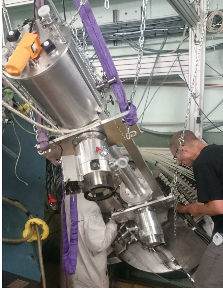
FIGURE 4.7: A photo of FiFI being mounted at the focal plane of Lohengrin.
