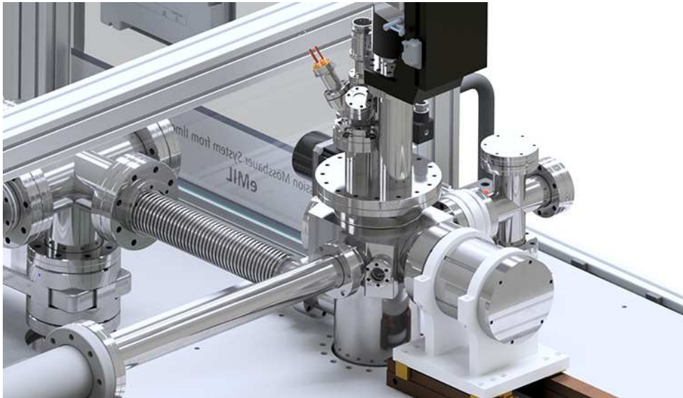
FIGURE 5.7: Quartz window, for light exposure experiments located next to the beam (through the GLM chamber) on the left and the Beryllium window on the right.
