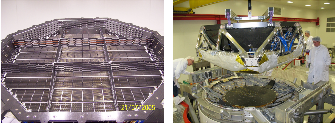
Figure 3.19.: Left: The partially assembled transition radiation detector [164]. The fleece radiator above the visible layer of tubes, as well as the four uppermost layers have yet to be installed. Right: The installation of the TRD on top of AMS [164].
