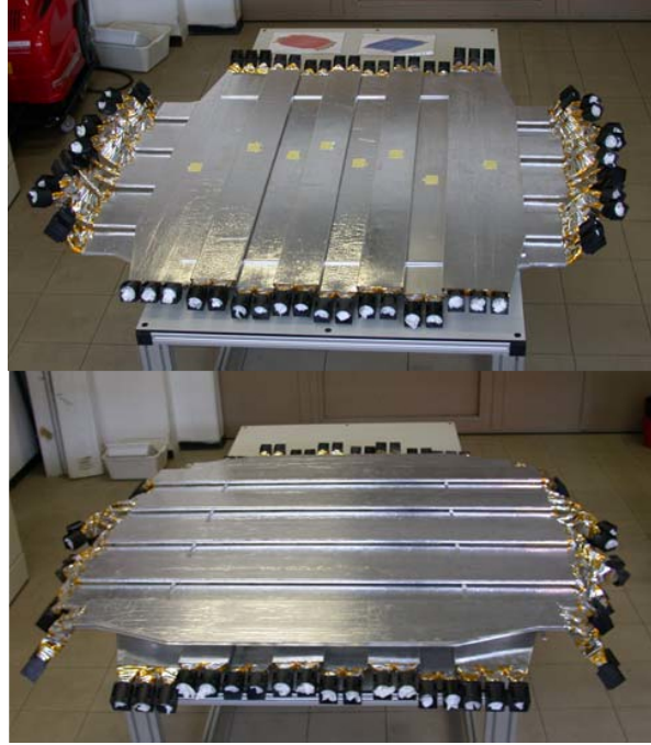
Figure 3.16.: The AMS-02 Time-of-Flight detector. The upper photo shows the two upper TOF layers, the lower photo shows the lower TOF system [154].
