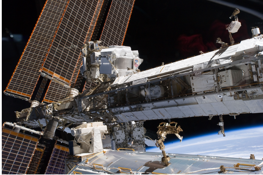
Figure 3.1.: The AMS-02 detector installed on the ISS [113].
