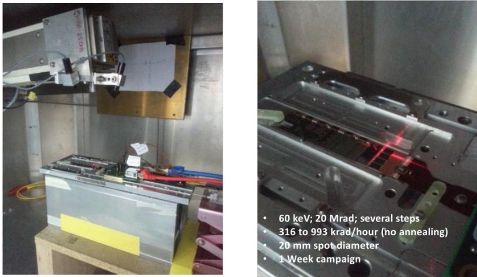
Figure 8.2: Setup of the irradiation measurements: The module was put in a 60 keV X-ray chamber and cooled with an aluminium cooling block and water chiller, all back-end electronics were put outside of the chamber.
