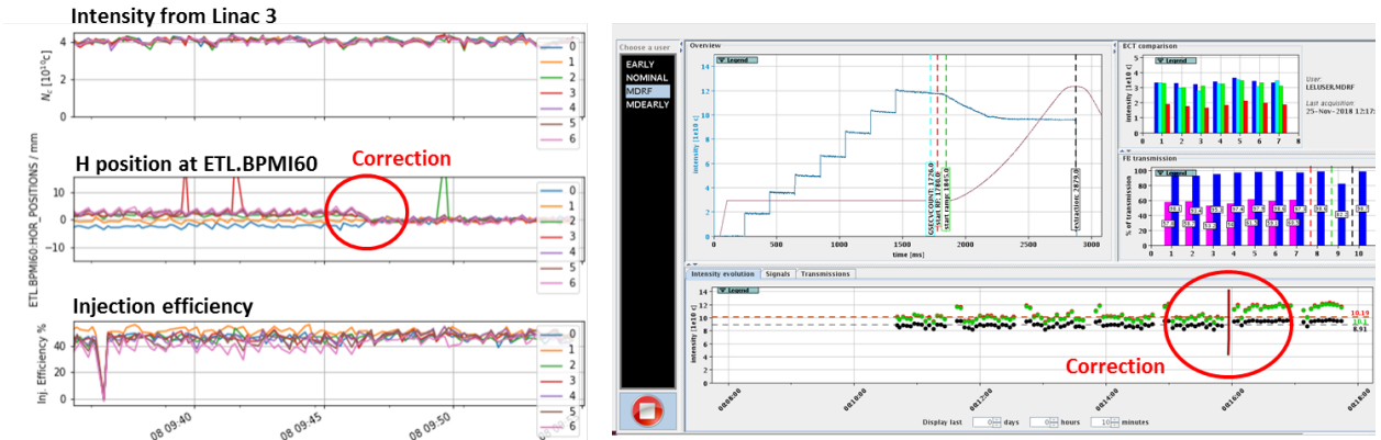
Figure 90: PS stray field correction using the injection equalizer. Left plot, intensity, horizontal position at the ETL.BPMI60 and injection efficiency for the 7 pulses sent from Linac 3; right plot, the “equalized” injection efficiency after the trajectory correction from the LEIR monitor application (see Fig. 3 for details on the LEIR monitor).
