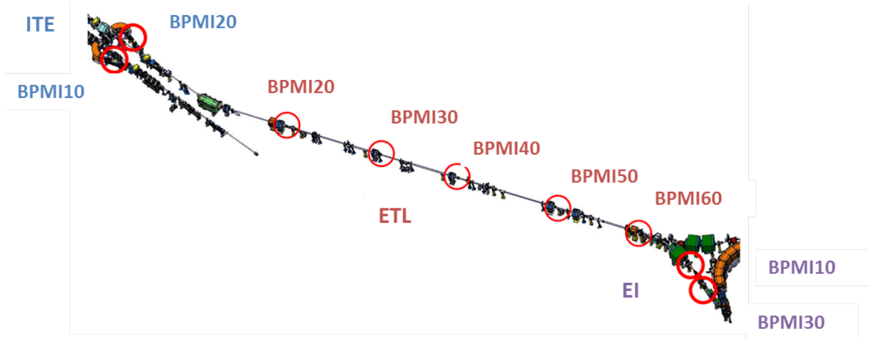
Figure 4: Nine new BPMs installed in the injection lines ITE (blue), ETL (red) and EI (purple) to allow a better trajectory measurement of the Linac 3 pulses injected into the LEIR machine (at the bottom-right).
