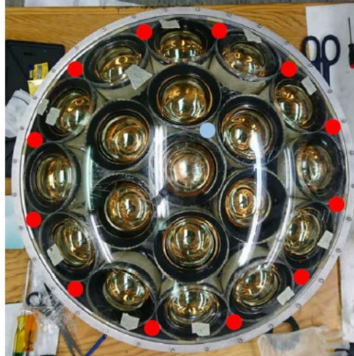
FIG. 30. Front-face of the mPMT showing the location of the pulsed LED (blue) and the constant LEDs (red).
