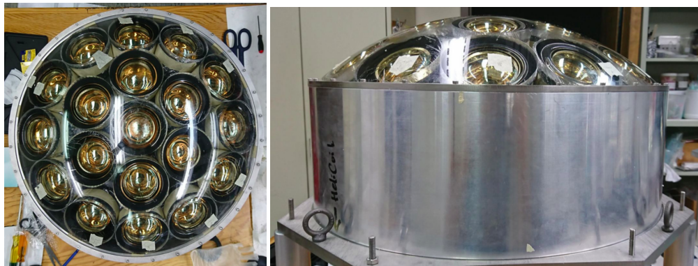
FIG. 25. Top (left) and side (right) views of the mPMT prototype.
