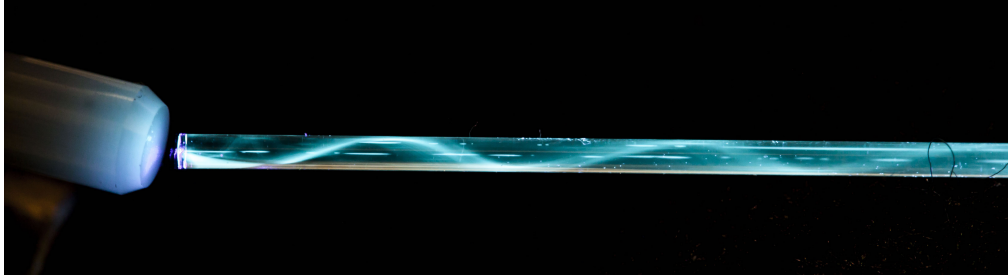
FIGURE 3.4: Picture of the propagation of a 406 nm laser beam 2 \mu\text{m} wide inside a silica-based optical fiber: the internal reflection phenomenon is clearly visible and various propagation paths are present in the first part of the fiber, depending on the injection angle of the laser beam.
