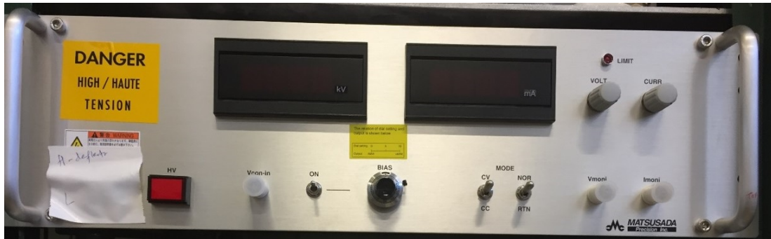
FIGURE 2.2: Static PSU for Deflector
