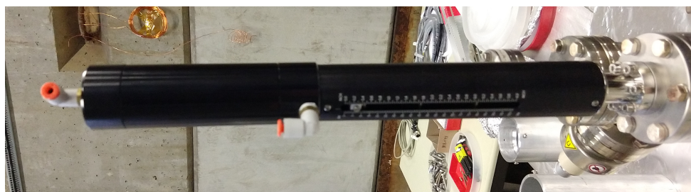
FIGURE 2.6: Piston connected to a Faraday cup in the vacuum tubing
