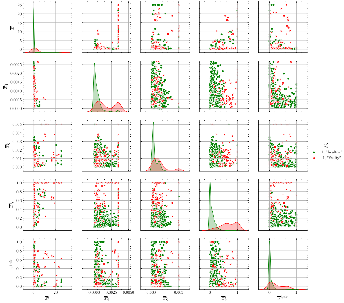
Figure 4.16: Distribution of the compressed QH current features \bar{x}^i .
