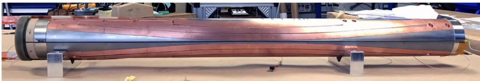
Figure 1.5: Picture of the 720 mm long HTS dipole coils Feather-M2.1-2, wound with ReBCO Roebel cable within the frame of the European EUCARD-2 collaboration [19]. The picture is taken from [55].
