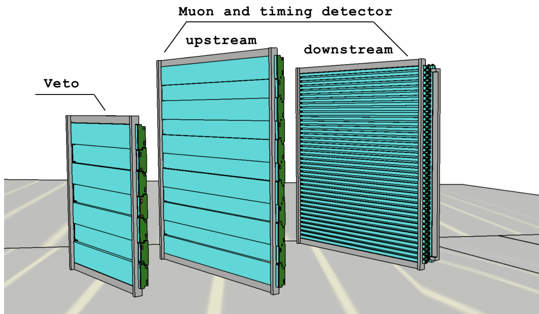
Figure 14: Layout of the upstream and downstream configuration of the muon and timing detector planes. The veto plane is also shown on the left side for comparison.
