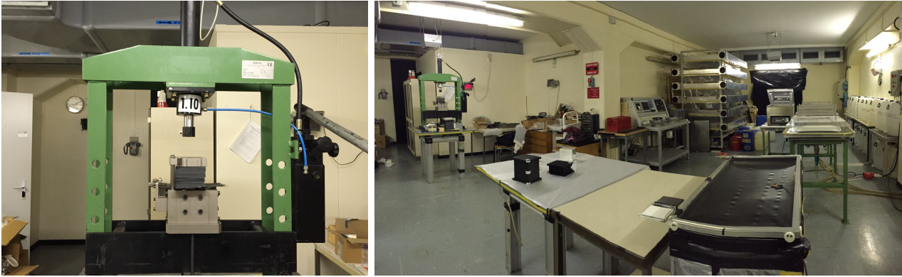
Figure 11: Left: press used in the emulsion laboratory at CERN to prepare the ECC target. Right: the SHiP emulsion laboratory at CERN.
