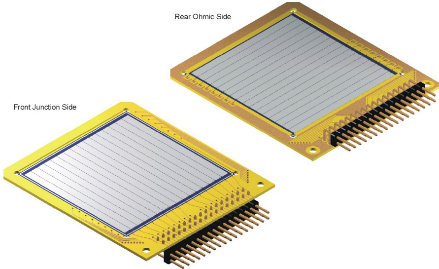
Figure 3.3: Picture of a W1 detector. The segmentation of the silicon is orthogonal on the two sides, effectively creating a number of pixels.
