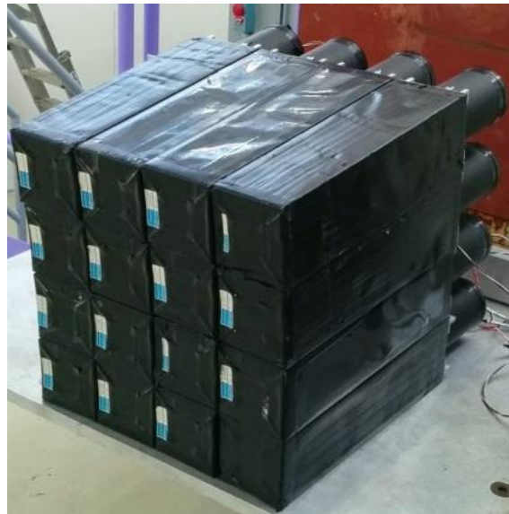
Figure 8: Stack of lead crystal calorimeters.
