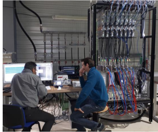
b) Test-stand for “accelerated ageing” of SSPA modules
