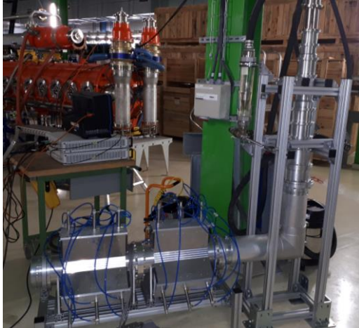
a) Set-up for RF short circuit tests
