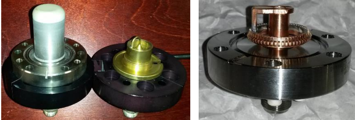
Figure 71: RF probes of LEP type with ceramic window (left) and new probes with coaxial feedthrough (right).
