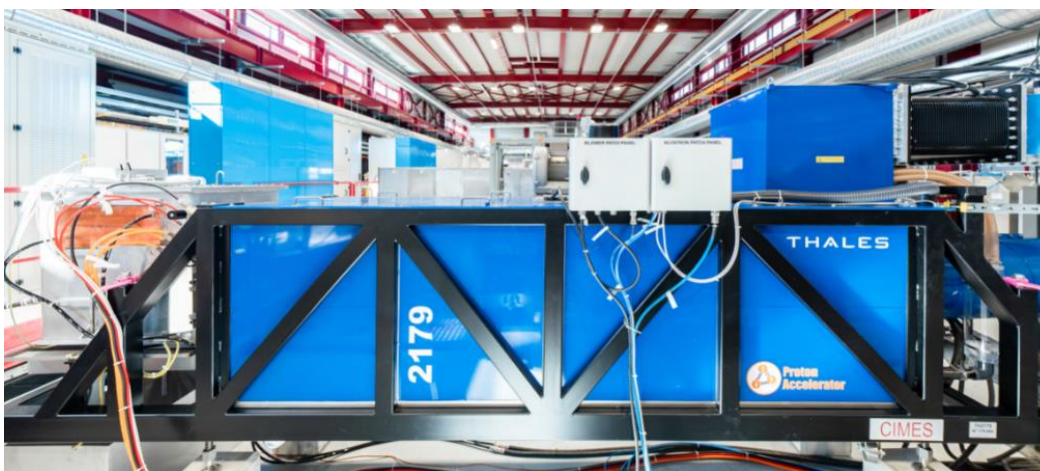
Figure 72: The new, state-of-the-art, Linac 4 klystron (Thales version), providing 3 MW at 352 MHz.
