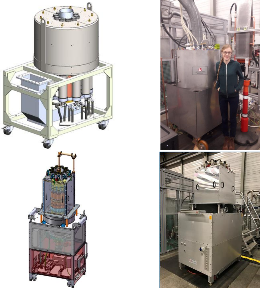
Figure 103: Top row: L3 MB-IOT; bottomrow: Thales/CPI MB-IOT. For both devices, the 3-D rendering (left) and a photo (right) of the device under test at CERN are shown.
