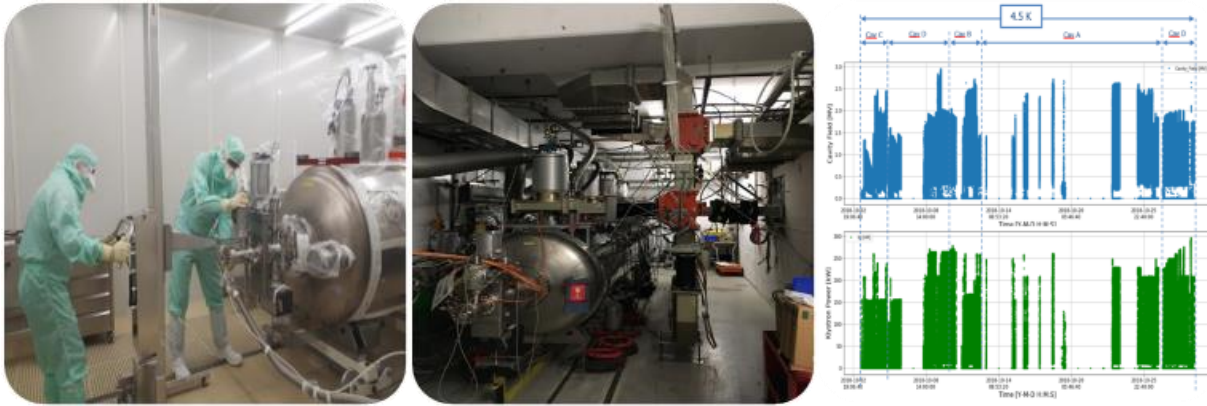
Figure 13: Left: Preparing ACS module “America” in the Clean Room; centre: “America” in the test bunker in SM18; right: test results demonstrating the reach of each cavity up to 2.3 MV.
