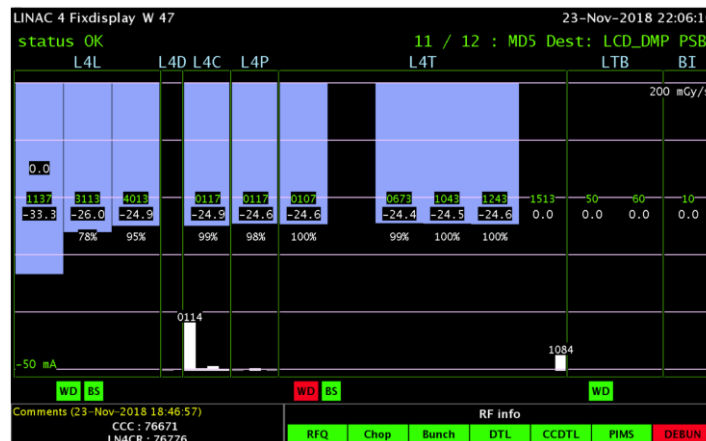
Figure 49: Linac4 current measured by beam current transformers from the source to the Linac4 dump.
