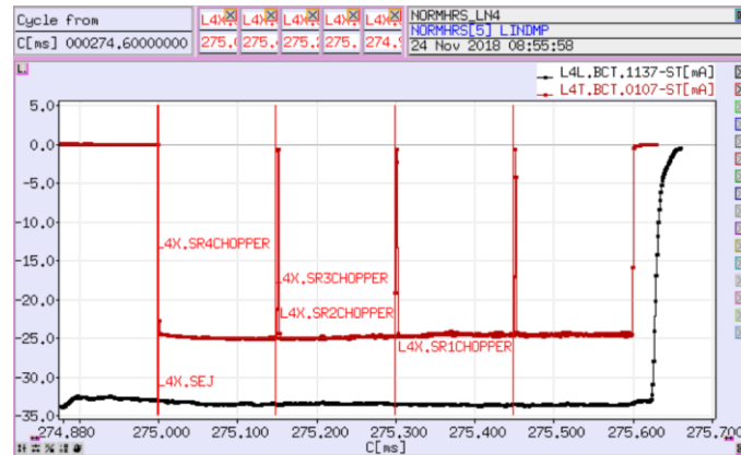
Figure 50. Linac4 beam current of 25 mA for each of the four PSB rings (red curve; 150 \mu s per ring)
