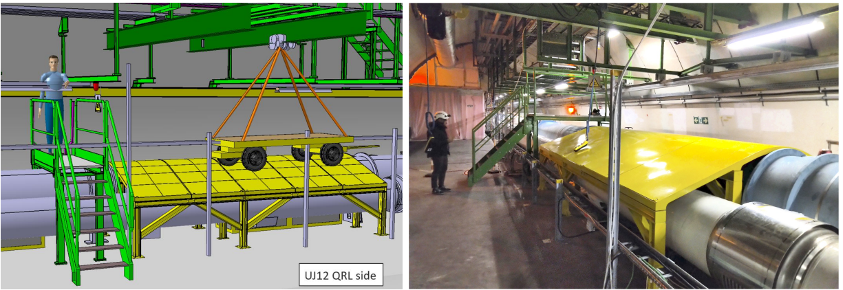
FIG. 24. The schematics of the transport setup at UJ12 (left) and a current photo of the site (right). The yellow QRL protection will allow us to transport FASER \nu even when the LHC is cold.
