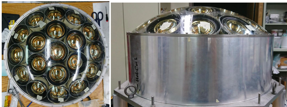
FIG. 12. Top (left) and side (right) views of the mPMT prototype.
