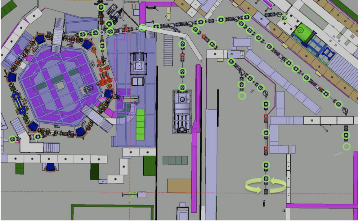
Figure 15 – Layout of ELENA facility indicating the positions of the 43 beam profile monitors which will be contributed by the ASACUSA collaboration.
