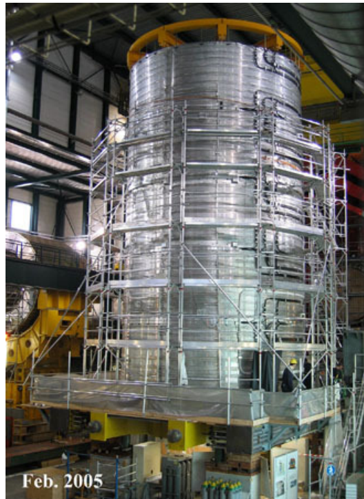
Figure 2.3: Coil of the superconducting magnet [2].
