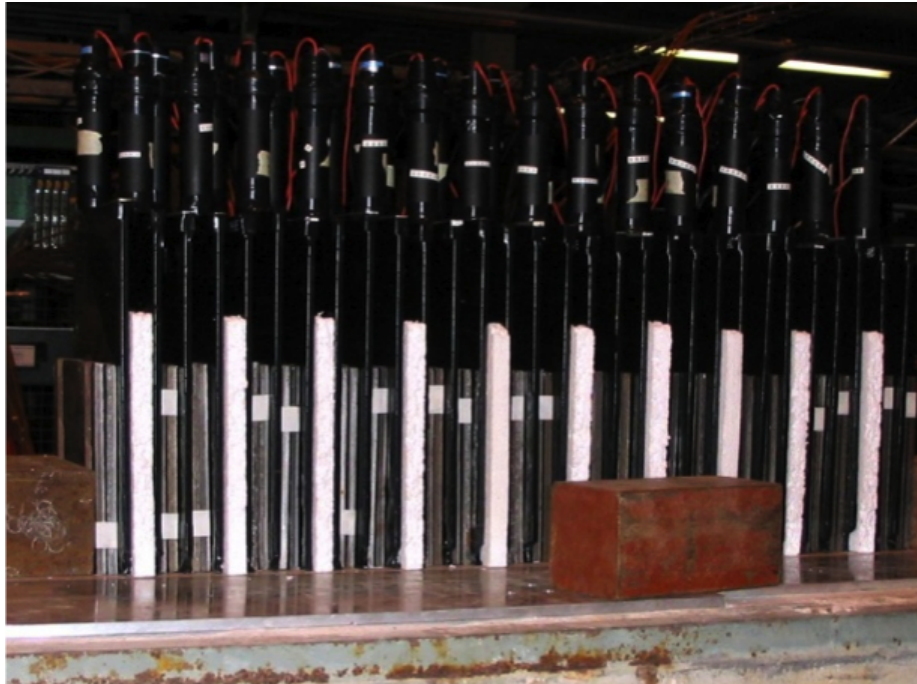
Figure 3.8: The calorimeter prototype in the electromagnetic configuration.
