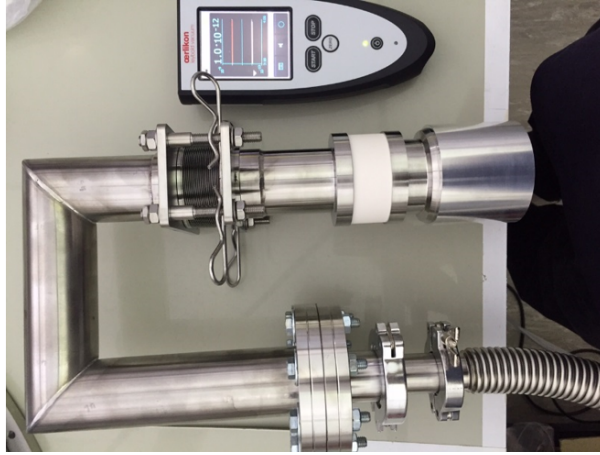
Figure 50: Replacement target pipe with mitre joints during helium leak testing
