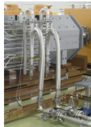
Figure 26: Quick-action water connectors.
