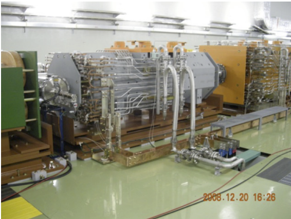
Figure 22: A whole view of PQ2 magnet, equipped with quick electric and cooling water couplers.
