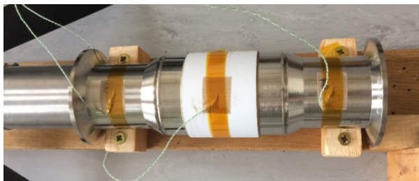
Figure 51: Brazed ceramic isolator during rapid cooling test
