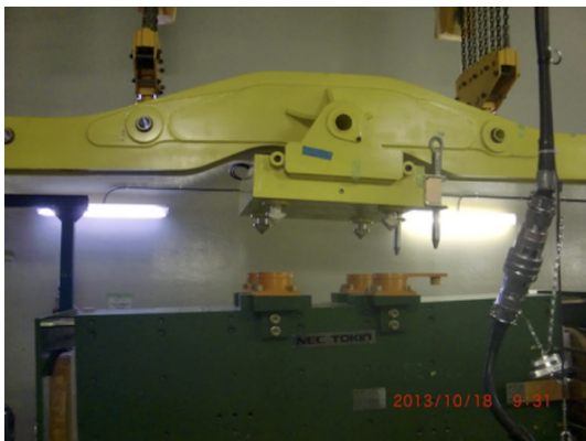
Figure 24: Twist-lock semi-remote hoisting attachment.
