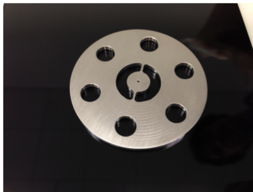
Figure 3.9: Ring aperture used to select a trajectory of a radius between 12 and 18 mm. The small hole in the center is for the Laser to pass for alignment. From [8].
