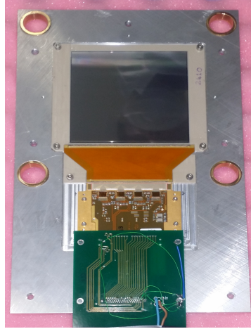
Figure 3.6: Sensor module hosting the silicon sensor, the pitch adapter and the front-end electronics.
