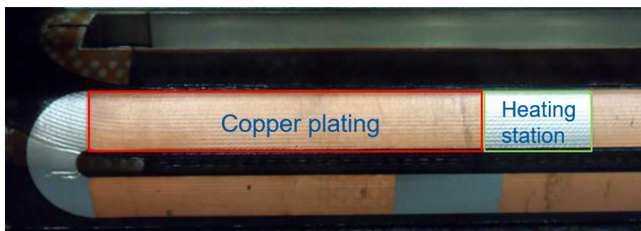
Figure 2.16: Picture of one quench heater strip. Used for high energy superconducting magnets [40].
