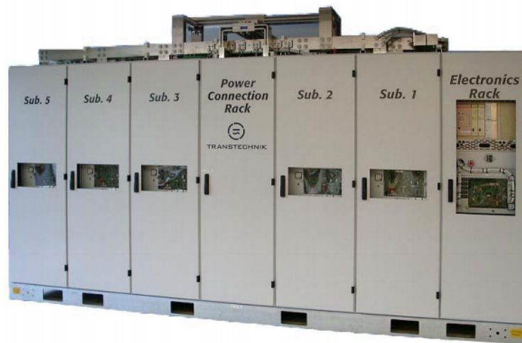
Figure 2.3: LHC main quadrupole power converter. Division into five sub modules and a power rack connection [28].
