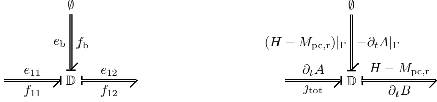
Figure 2.28: Bond graph representation of a Stokes-Dirac structure.
