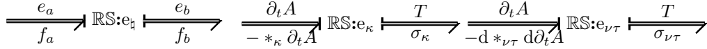
Figure 2.32: Bond graph representation of an RS source for eddy (middle) and coupling (right) currents.
