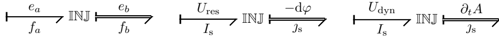
Figure 2.24: Bond graph representation of a multiport injector relating lumped and distributed voltage and current for resistive (middle) and inductive (right) components.
