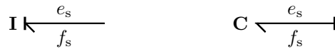
Figure 2.12: Bond graph representation of an I-type (left) and C-type (right) storage in preferred (integral) causality.
