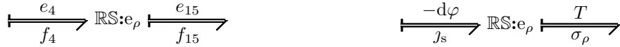
Figure 2.31: Bond graph representation of an RS source that relates electric and thermal domains.
