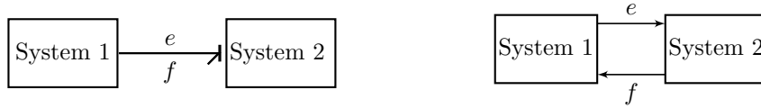
Figure 2.2: Representation of power exchange between two systems by means of a word bond graph (left) and a block diagram (right). Note that the block diagram does not indicate the direction of the power flow.
