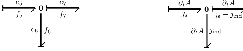
Figure 2.25: Bond graph representation of the 0-junction (2.83) representing distribution of the source current density J_s .
