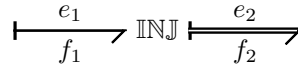
Figure 2.18: Bond graph representation of a multiport injector mapping a lumped bond into a distributed one.
