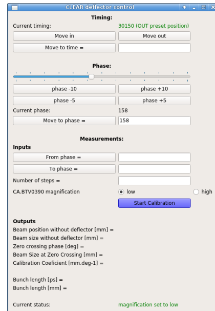
Figure 2.5: Graphical interface of the deflecting cavity control panel in its most recent version (summer 2018).
