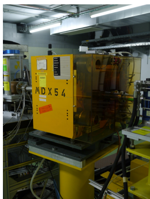
Figure 3.1: Dipole located at the end of the beamline, deviating the beam to the in-air experimental line.
