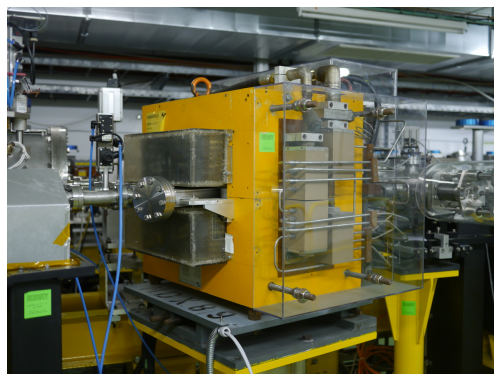
Figure 3.2: Dipole located at the end of the LINAC, deviating the beam to the VESPER experimental line.
