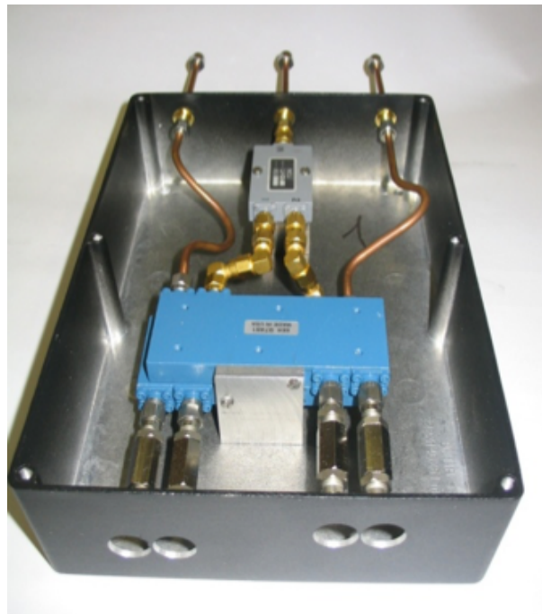
Figure A.1: CLEAR cavity BPMs first part of the electronic hardware: hybrid coupler and combiner.
