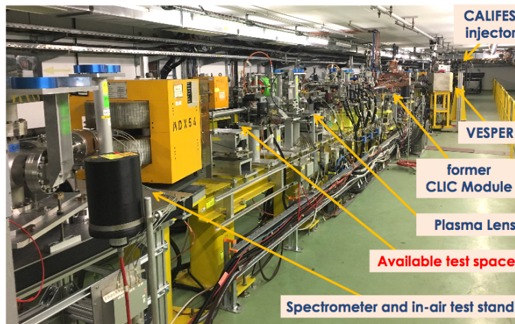
Figure 1.4: Picture of the CLEAR beamline (November 2017), captioned from the end of the line. (credit: Bruno Cassany)
