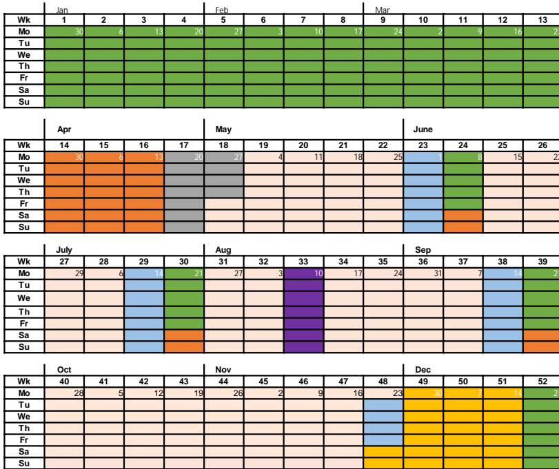
Figure 4.9: An idealized LHC schedule based on [37]. Green color signifies technical stops, orange commissioning, gray scrubbing, beige proton physics, blue machine development, violet special physics, and yellow ion physics.
