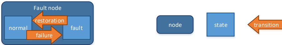
Figure 8.2: A fault node in the OpenMARS contains a Markov model with fault and normal states and transitions between them [2].
