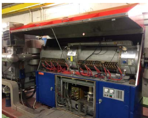
Fig. 3. CERN PS Ferrite-loaded Cavity driven by the tube amplifier. A feedback amplifier is used for beam loading compensation and higher gain is required to cope with larger intensity.
