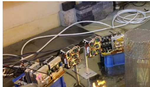
Fig. 10. Irradiation test of solid-state amplifiers (left) at QST-Takasaki. The 60 Co source will be inserted in the tube of wire mesh (right). The other setups for MOSFETs test are also shown
