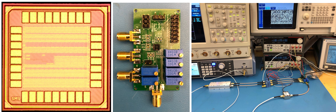
Figure C.5: The ADC chip, test board, and test setup.
