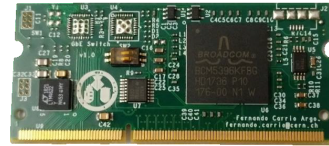
Figure 5: Picture of the TileCal GbE Switch mezzanine card.
