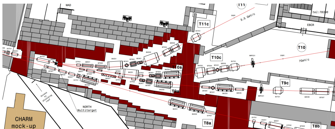
Figure 9.1: Partial illustration of the East Hall. The T10 and T11 beams are entirely visible, while the T8 and T9 beams extend further downstream. [36]
