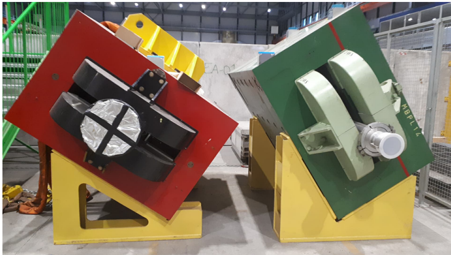
Figure 7.1: Placement of the MBPL magnets on their support in H2-VLE (left) and H4-VLE(right).
