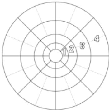
Figure 3.6: Layout of the VZERO silicon rings.
