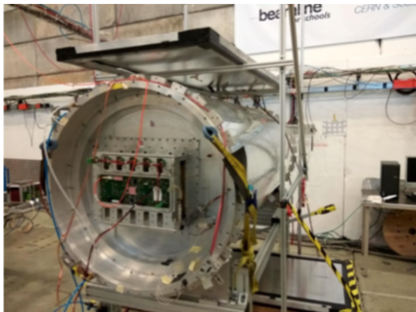
Figure 3.33: The experimental setup during the TPC test beam in T9 at CERN. The Micromegas MM0 is mounted on the HARP field cage. Two alluminium boxes containing plastic scintillator bars read out by SiPM are positioned on the top and the bottom of the field cage in order to select through going cosmic rays.
