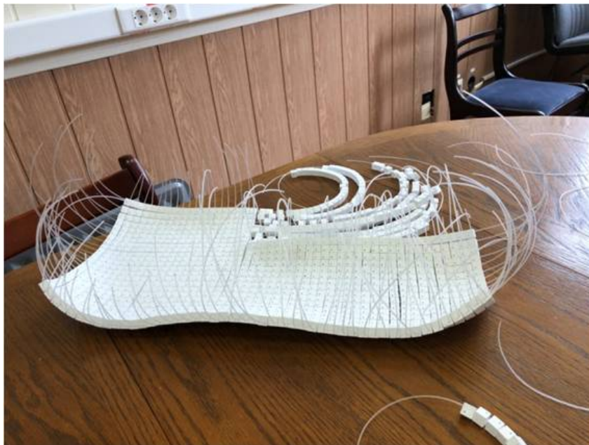
Figure 2.7: A plane of scintillator cubes formed with fishing lines
