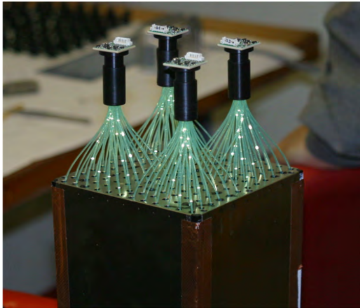
Figure 2.2.12: Photograph of an individual EMCAL module comprising four towers. The Shashlik WLS fibers that penetrate the module longitudinally are visible [36]
