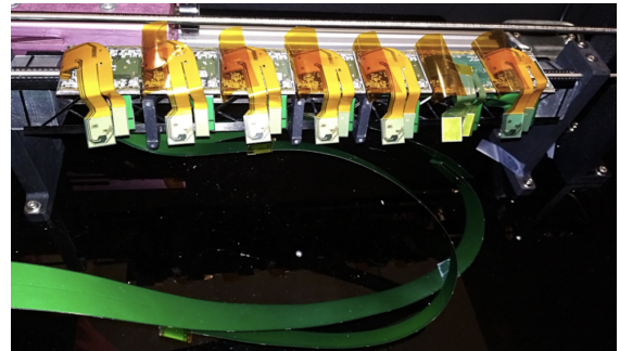
Fig. 1. A prototype developed for the central OB pixel tracker with seven quad pixel modules mounted on a carbon support including titanium cooling pipes. Powering is conducted as one serial powering chain and including the serial powering protection chip.
